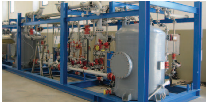
PFA/PTFE lined pumps and valves in a skid-mounted electrolysis system
